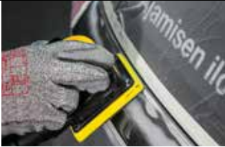
Paint removal and Feather edge sanding
