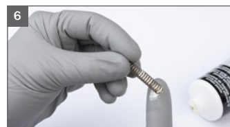
6 Grease and insert paint needle spring
