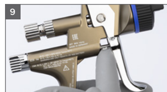
9 Grease visible part of air piston rod
