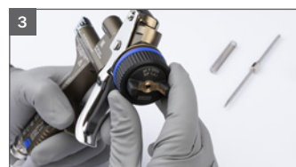
3 Assembly of the air cap
